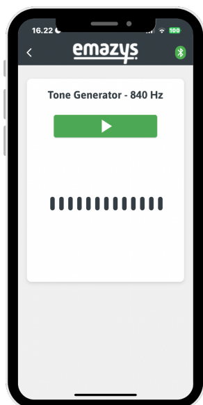
Figure 2: Testing principle of the tone generator function. The Z300 PVT transmits frequencies into the PV system. These tones are picked up and amplified by a handheld tone pickup device. This helps locate disconnections or trace wiring.
